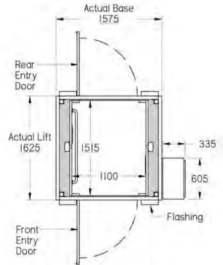
B MODEL - Dual Car Entry Elevation
